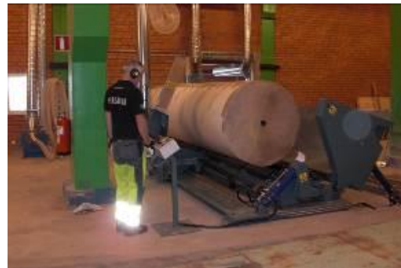
Smurfit Kappa – Roll Saw with roll loader
