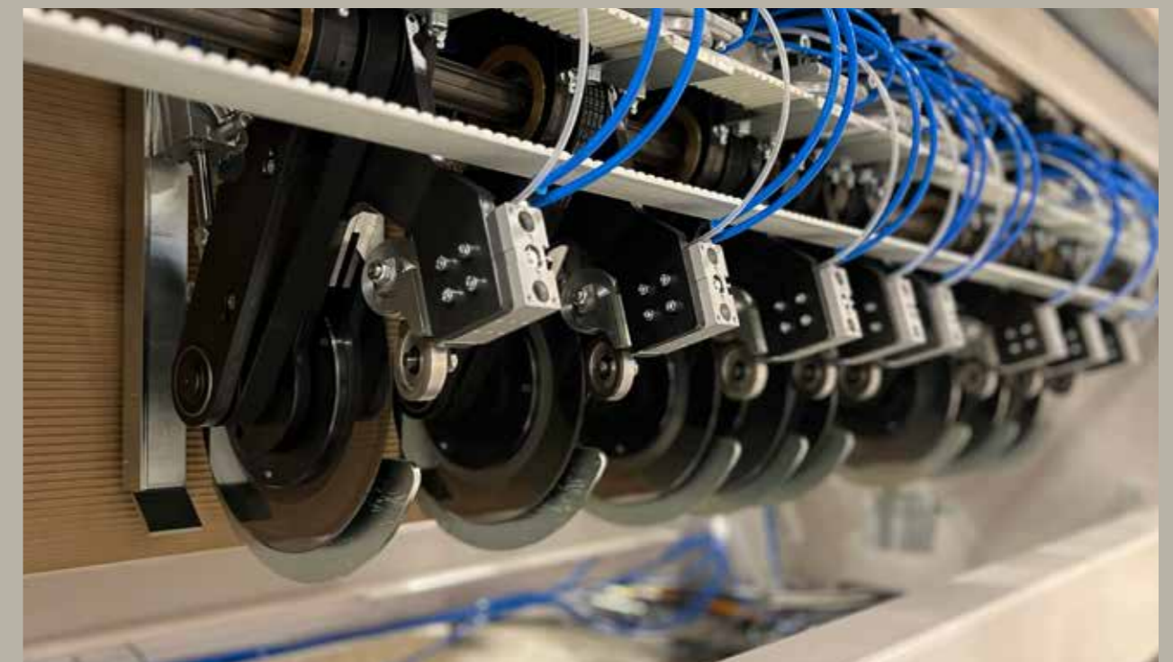
Sharp cuts through easily adjustable longitudinal cutting knives with automatic knife sharpening.
